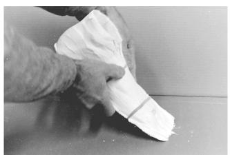
The first pour is about 1/3 capacity of the shell. The shell is tilted and shook so the toe area fills without bubbles.
