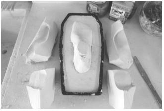
The top of negative cast has been separated. The inner cast (which is a cast of a last) is ready to be removed.
