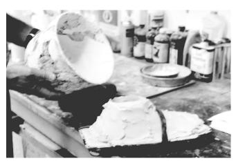
The plaster is being poured into the negative cast.
