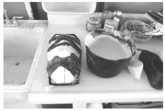
The negative cast is full of plaster. It needs to dry a couple of hours.
