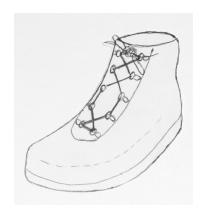
Double lace wrapping, which can be used to have one area of laces either tighter or looser.
