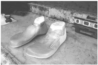
The inserts and lining have been added. The single knit sock has been added, latexed and the top front of the sock cut away. These are going to be soft shoes.
