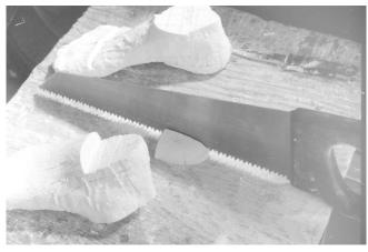
6 Using a drywall saw to narrow the heel piece. If necessary, make two cuts depending on the thickness of the blade and the desired amount of narrowing.
