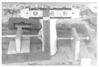
1 Here are some simple tools I built to hold up casts when checking vertical alignment etc. Sometimes little wedges under the soles of casts are not enough.
