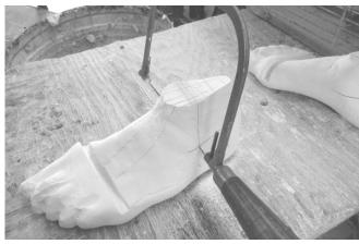
12 Another heel narrowing, but this time the whole heel is narrowed. Therefore, the saw cuts all the way through the casts.
