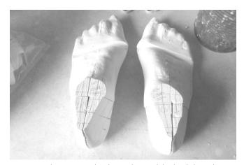
The casts are back together and the heels have been narrowed.
