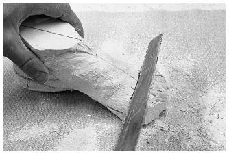
16 An angled vertical cut is made down to the horizontal cut.
