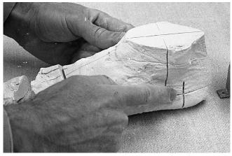
37 These are press cements. Which means press when the cement is wet and hold. If you want to use a contact cement, then you have to wait for it to become tack free before sticking together.
