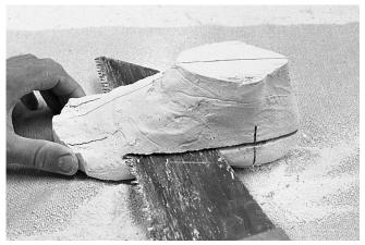
15 The front of cut is just to the rear of the bunion (big toe) and tailors (little toe) joint.
