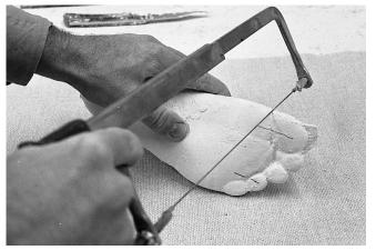
6 Using a spiral wire saw blade to cut the toes off. A 10pt coping saw blade is a good alternative.
