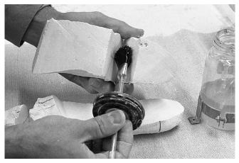
34 Putting glue on the parts; either rubber cement or a vinyl adhesive.
