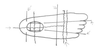
The arrows point to the pencil marks which must be aligned. Notice that the top pieces have been lowered the width of the saw cut. The front top piece has moved backward the width of as many vertical saw cuts as have been applied. Therefore, there is a gap at the front of the top piece which must be filled later. The front semi-vertical cut was made behind or to the rear of the mid point of the bunion joint. The back pieces at the heel should match flush.
