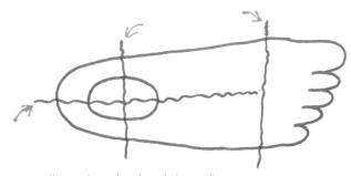
Arrows point to squiggly lines which represent saw cuts usually made with a hand dry wall saw.
