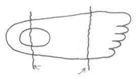
Arrows point to squiggly lines which represent saw cuts usually made with a hand dry wall saw.
