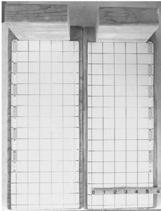
1 Measuring boards for measuring length of feet. Measure and record each foot.
