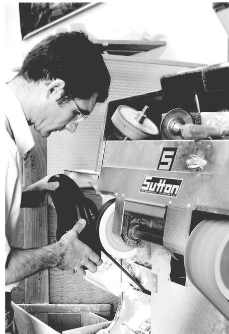
The concentrating craftsperson is sanding the underlap leather of a shoe in the "making".
