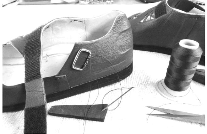
142 Usually a short piece of leather is used for attachment of the rectangular rings and a rivet is used to secure the leathers. But, for softness, the top ring is being hand sewn into place.
