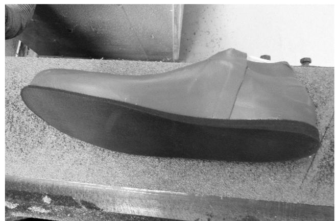
116 The ball to toe angle is sanded carefully on the flat belt sander to make sure it conforms to an even thickness. The transition area from toe to ball and ball to heel must be level and uniform so that it will be beneficial to the wearers gait.
