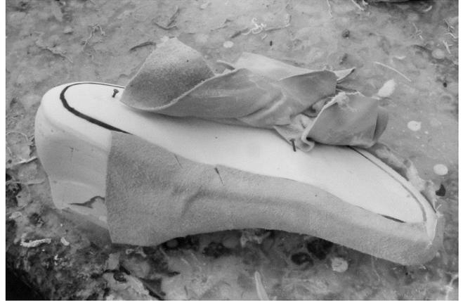
10 The excess lining leather is being removed from inside of the underlap line.
