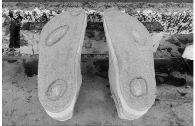
82 A view of the finished bottoms. The extra sock materials on the tops was removed before leathering. Both sandals were made to match.
