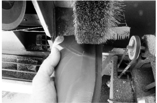
124 The lower sides of sandal are lightly brushed to remove unwanted dirt and glue on the leather above the attachment seam.
