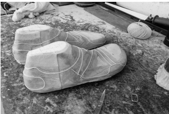
25 The design cord is attached to the lining leather. The artisan and/or craftsperson selects and refines the placement of the design cording with a lot of thought about what is desired in the attributes of the finished sandal design.
