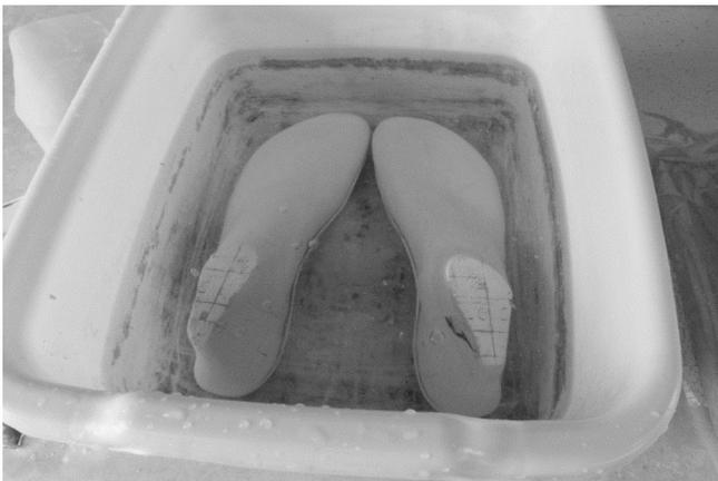
5 The lasts with inserts attached are soaked in water one to two minutes.
