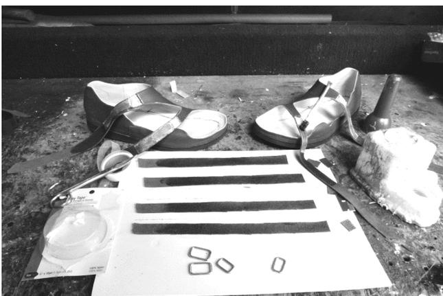
139 Glue is being applied to the inside of the straps after being applied to the under side of Velcro®. When the glue is dry, the looped Velcro® will be pressed on to the straps.
