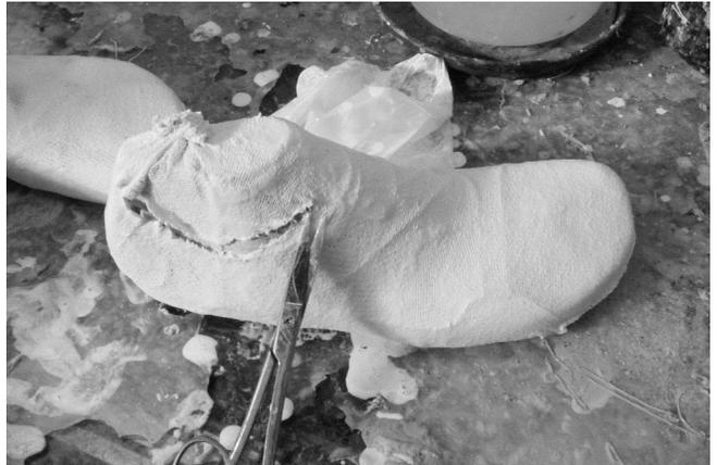
36 While still wet, the excess sock is removed above the upper design cord.
