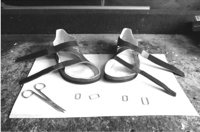
141 The Velcro® has been trimmed to fit the leather of the straps and the square "D" rings.
