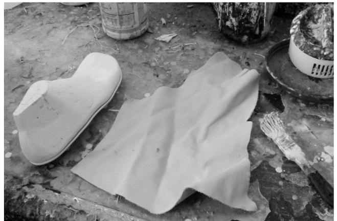
6 The wet last and front lining leather are ready. The lining leather is smooth side up.
