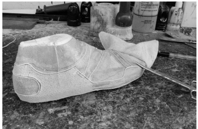
38 Usually the sock is cut out to the design cords and a Monks Cloth heel counter may be added. This pair of sandals will be soft so no heel Monks Cloth counter is added and the front of sock is being removed.
