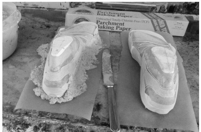
50 The "mud" voids are filled and the "mud" is pressed into the last and pulled up making a uniform edge with a lot of excess because the "mud" will shrink as it dries.
