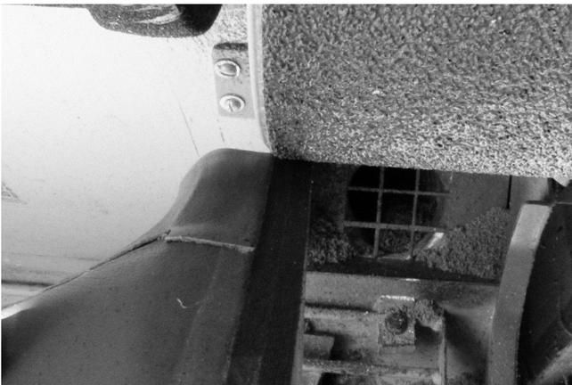
113 The mid sole and heel wedge are rough sanded around outer edge.
