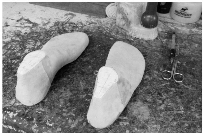
20 Top view of fully leather lined lasts.
