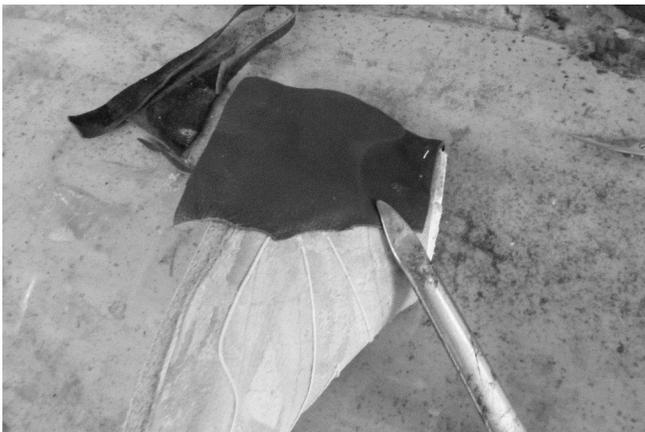
89 The leather at design cords is pressed with a modified butter knife which was made blunt and rounded with a slight bend at tip.
