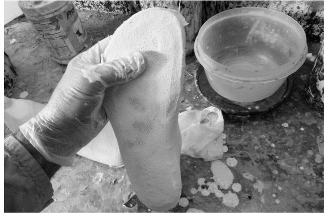
34 The latex is rubbed into the fabric and the excess is squeezed out.
