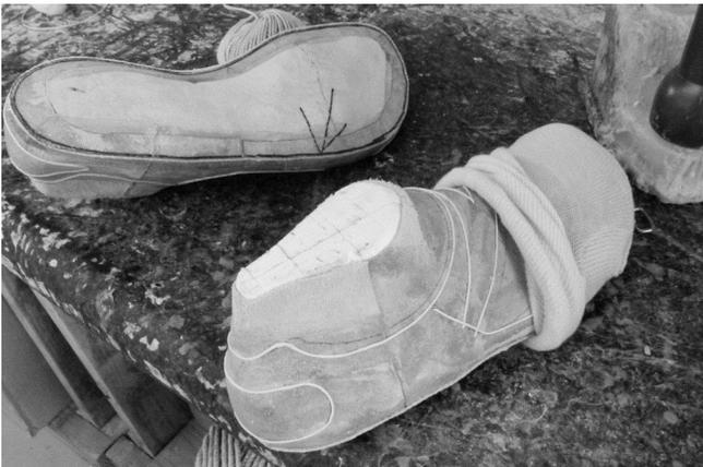
29 A double knit sock is added. Sometimes a single knit sock is used. And, sometimes no sock is used. The consideration of softness, strength and durability depends on the needs of the customer.
