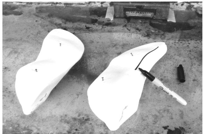
2 An underlap design line is being marked.
