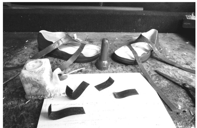
140 Glue has been applied to the underside of the hooked Velcro® and area of attachment of outer leather. When the glue is dry, the hooked Velcro® will be pressed into place and any excess glue will be immediately rubbed away.
