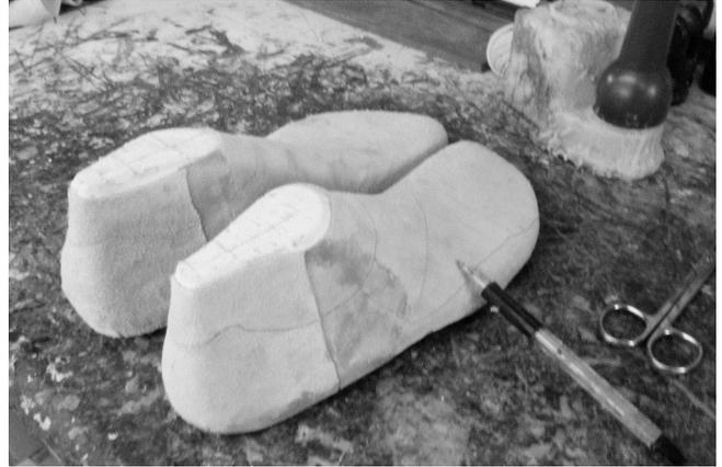
22 A pen is used to roughly mark the design of top of sandal.
