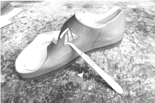
137 The internal designs are cut out with a #12 surgical knife.
