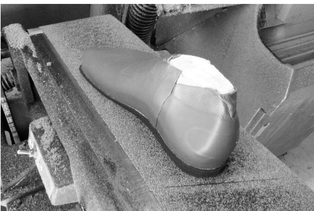
115 The taper is sanded flat from heel to ball and the levelness from medial to lateral is checked many, many times during the sanding process.
