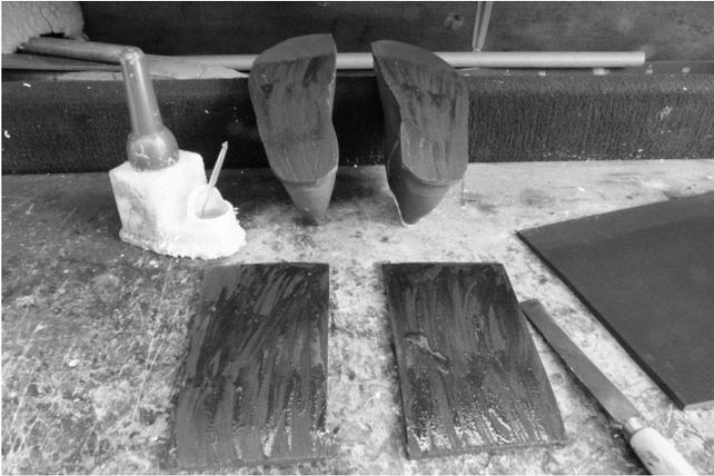
111 Glue is applied to mid sole from ball to heel and to 18 iron (3/8") heel wedge. Normal heel wedges can be 30,24,28 or 12 irons, sometimes 36.
