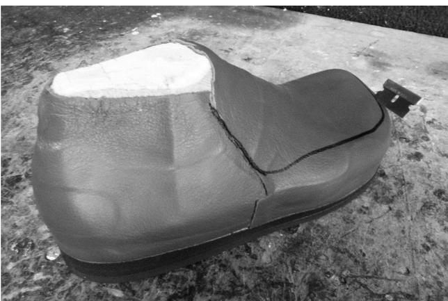
127 A razor blade is used to cut an opening.
