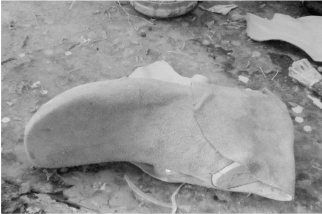
15 The heel lining leather is stretched and pulled and pressed onto the last and insert.
