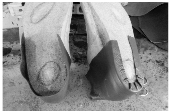
92 Glue is drying on the left and the underlap has been folded on the right.
