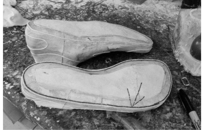
28 An outer bottom edge cord design is placed where the artisan wants the edge of the finished "mud" to be located.
