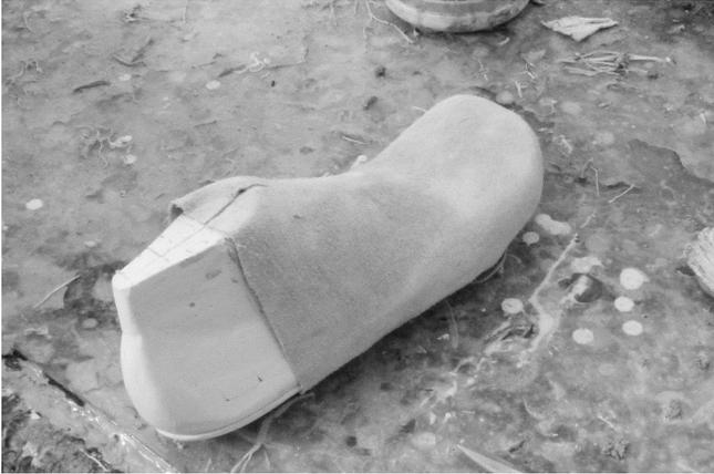
9 The lining leather is stretched and pulled and pressed until it is bonded to the wet last. Sometimes a little more fresh latex is need.
