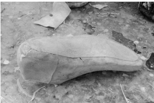
19 The bottom lining leather is cut at edge of underlap.
