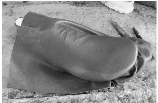
96 The leather is pulled, stretched and pressed around the toe box.
