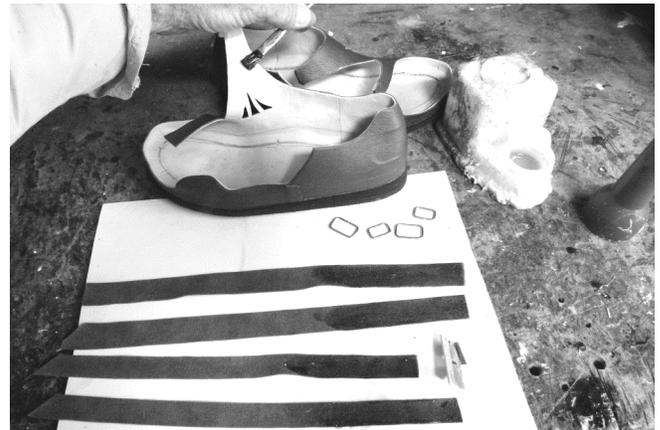
138 Glue is being applied to strap attachment area of lining leather and end of strap. When the glue has dried, the straps are attached and pressed.
