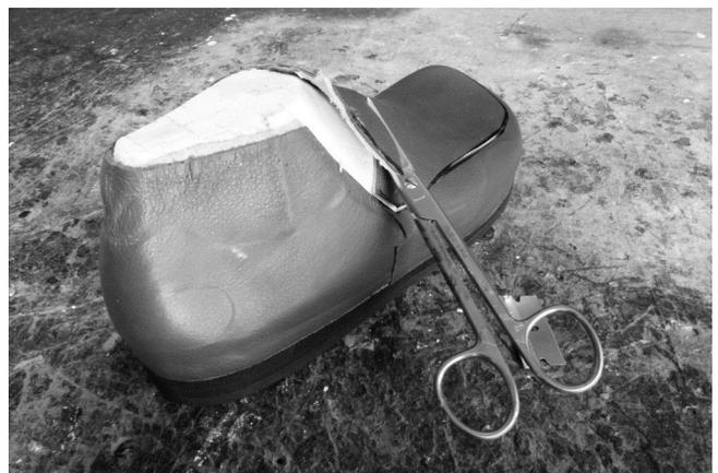
128 The excess leather at top of last is cut away. The last is lifted out in one piece. All the extra leather beyond the design cords is cut away.
