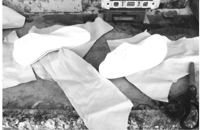
4 The lining leather is selected and cut to the desired size.
