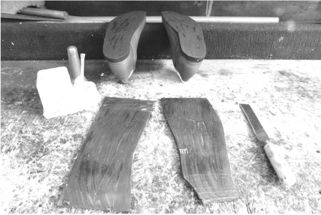
117 The finished mid sole, heel wedge and outer sole are glued.
